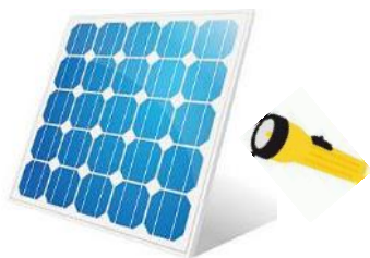
Illumination from rear to reveal cracks in the inner layer
